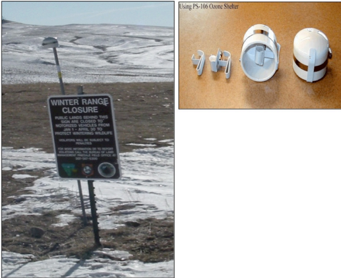
Figure 2-3. Ogawa O3 protective shelter mounted on gray PVC pipe and an Ogawa O3 ambient air passive sampler.
